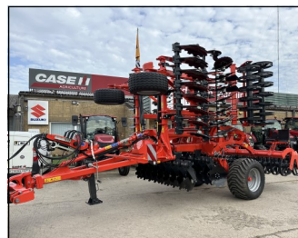
New Kuhn Optimer L 6000, 6m trailed disc cultivator, harrow, 600mm roller, brakes, front depth control wheels. £POA
